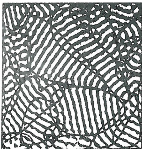
Figure 6: Striped roll patterns with dislocations from an experiment with chlorite-iodine-malonic acid reaction [Reproduced by kind permission of Q Ouyang and H Swinney]
