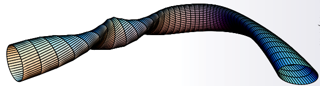
The geometry of a curved quantum waveguide. The effects of twisting and bending are demonstrated at the left and right respectively.
