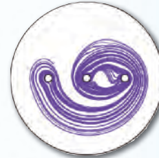
Material line pattern for a three-braid 'pseudo-Anosov' mixer after three periods (courtesy SE Tumas and J-L Thiffeault)
