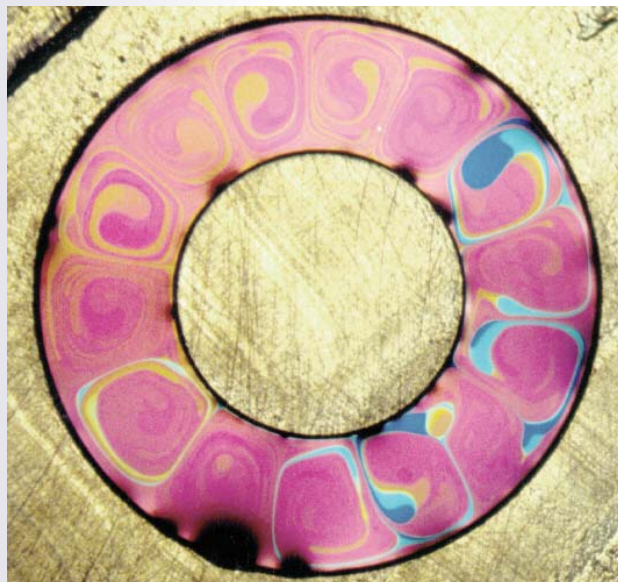
Electroconvection pattern formed in an annular smectic liquid crystal film. Colour variations correspond to local variations in film thickness
