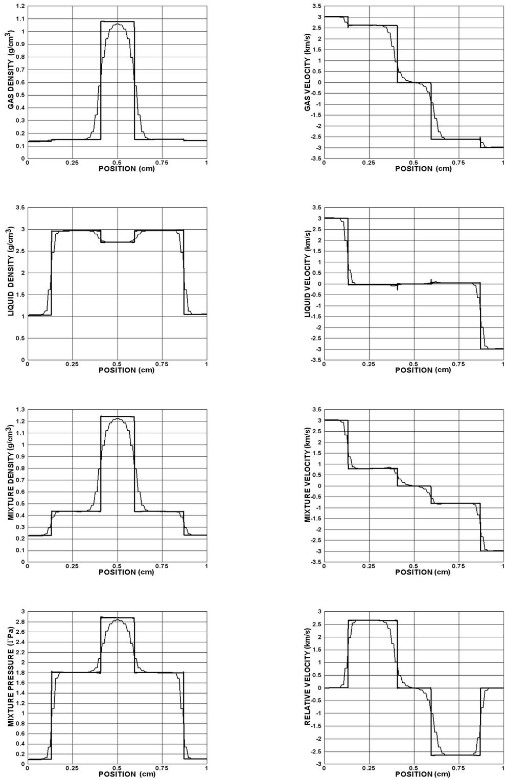
Figure 6: Test 2. Four-shock test problem. Reference solution (thick line) and numerical solution (thin line) obtained by the Lax-Friedrichs method for 100 mesh cells.
