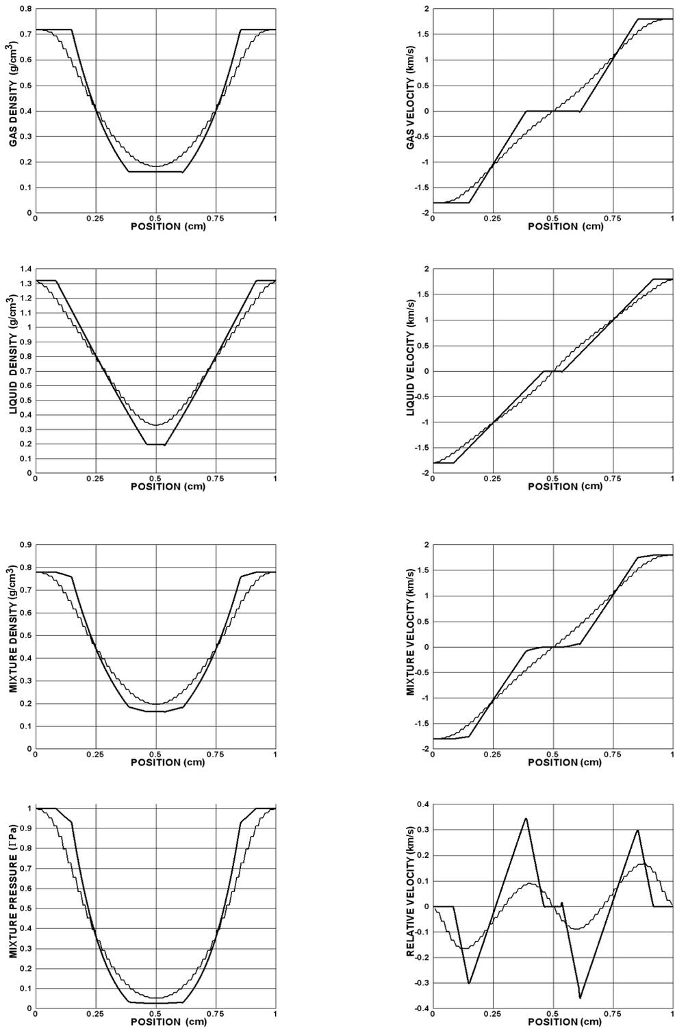
Figure 2: Test 1. Four-rarefaction test problem. Reference solution (thick line) and numerical solution (thin line) obtained by the Lax–Friedrichs method with mesh of 100 cells.
