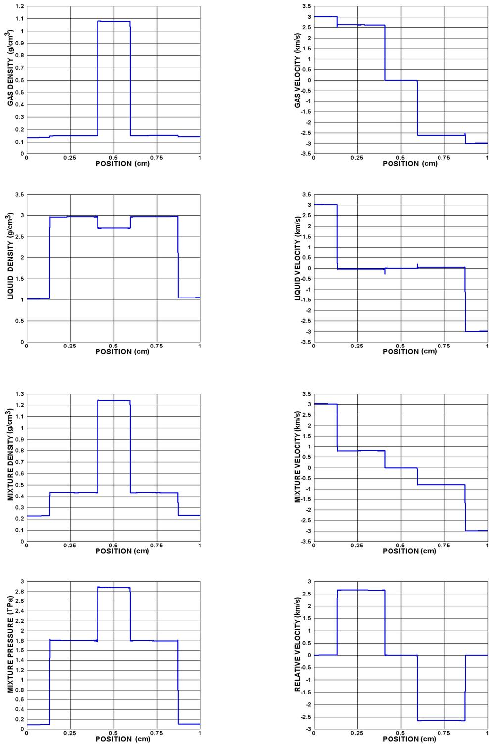
Figure 5: Test 2. Four-shock test problem. Reference solution using SLIC, SUPERBEE limiter and mesh of 4000 cells.
