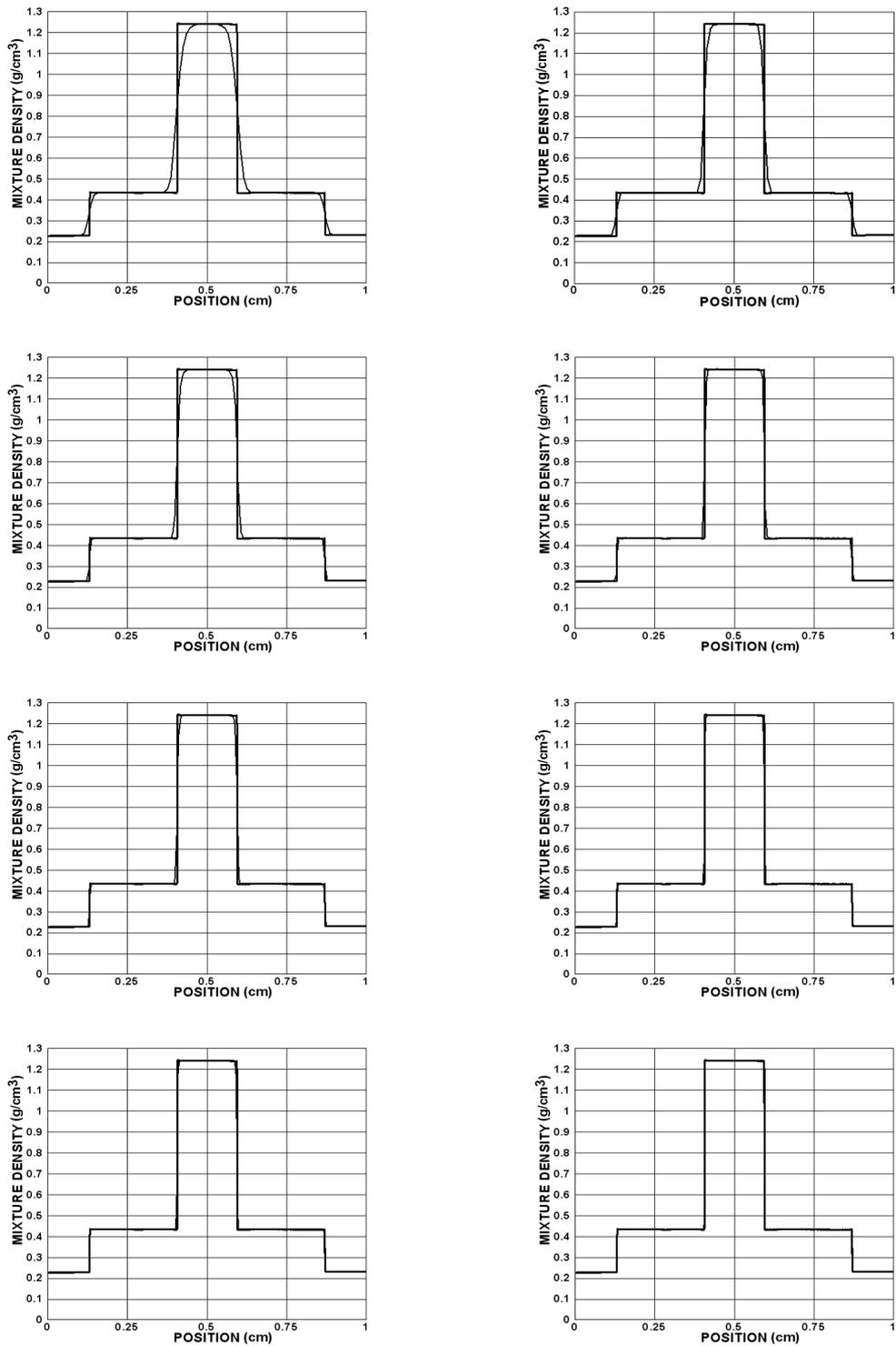
Figure 9: Test 2. Numerical convergence of mixture density for 4-shock waves Riemann Problem. Reference solution (thick line) and numerical solution (thin line) obtained by the FORCE (left column) and SLIC (right column) methods with meshes of 100, 200, 400, and 800 cells.
