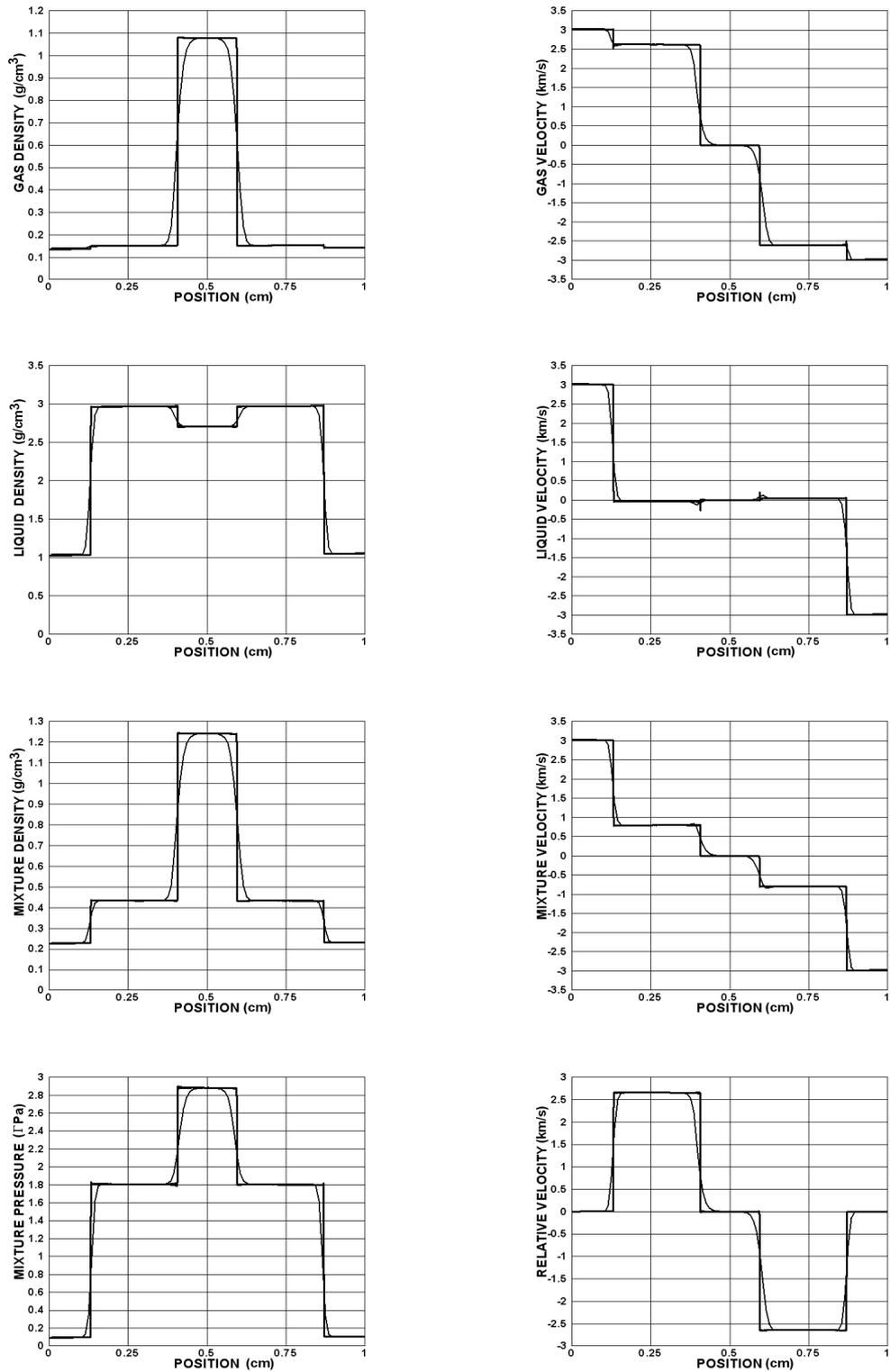
Figure 7: Test 2. Four-shock test problem. Reference solution (thick line) and numerical solution (thin line) obtained by the FORCE method for 100 mesh cells.
