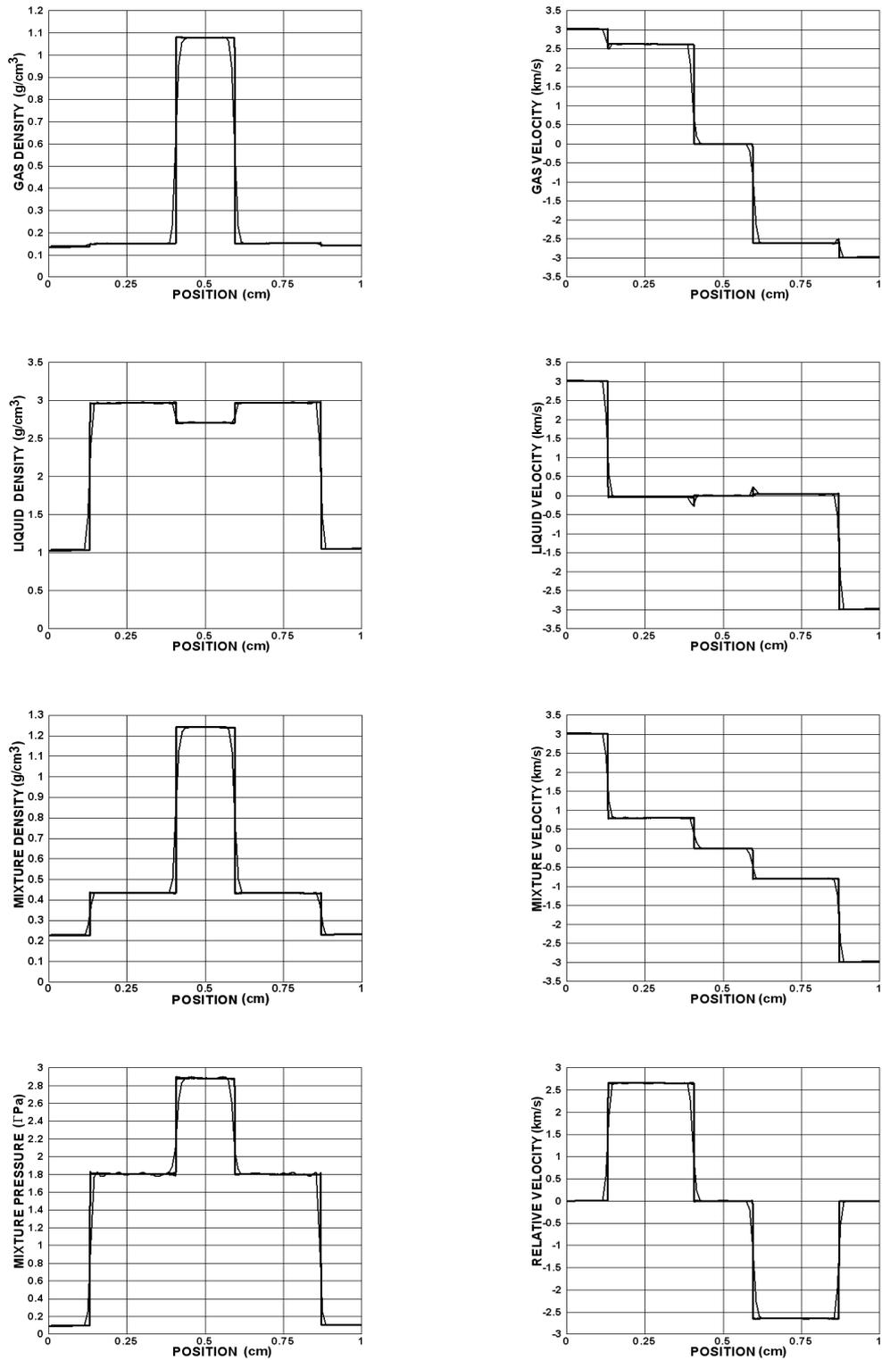
Figure 8: Test 2. Four-shock test problem. Reference solution (thick line) and numerical solution (thin line) obtained by the SLIC method for 100 mesh cells.
