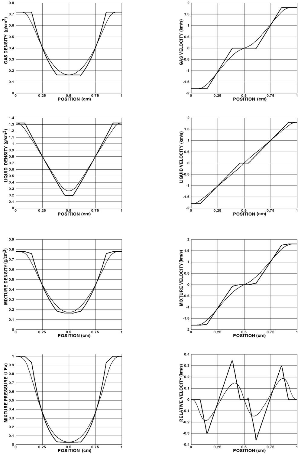
Figure 3: Test 1. Four-rarefaction test problem. Reference solution (thick line) and numerical solution (thin line) obtained by the FORCE method with mesh of 100 cells.
