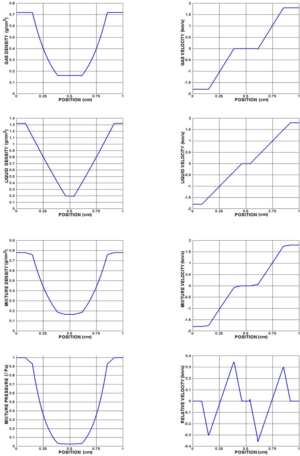
Figure 1: Test 1. Numerical results for 4-rarefaction waves Riemann Problem for 4000 mesh cells, TVD method, SUPERBEE limiter.
