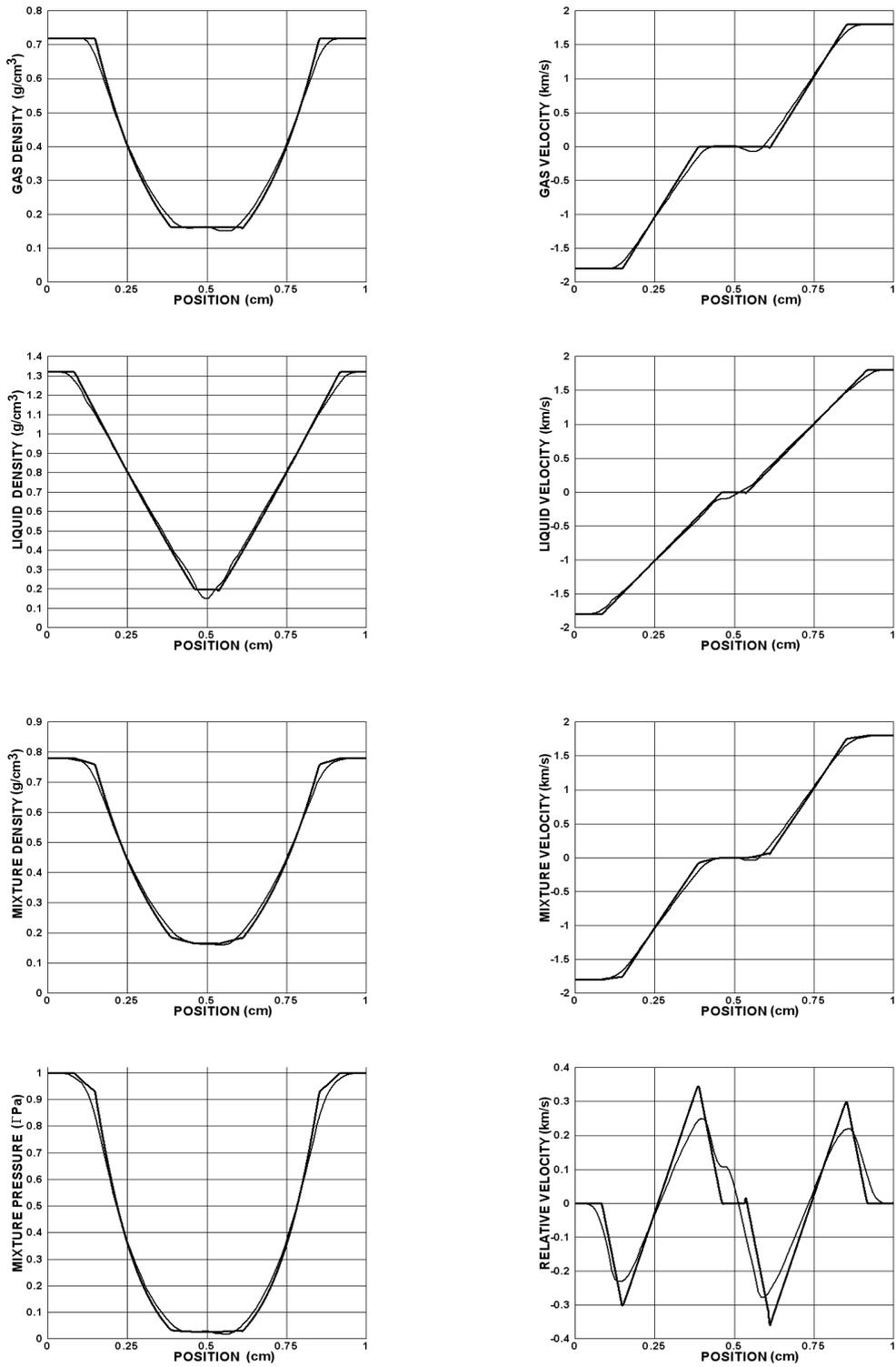
Figure 4: Test 1. Four-rarefaction test problem. Reference solution (thick line) and numerical solution (thin line) obtained by the SLIC method with mesh of 100 cells.
