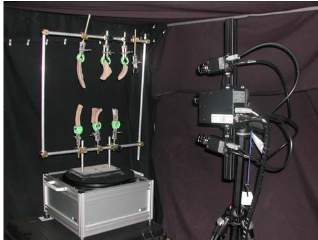
Figure 2: The scanning system (right) and a frame, with 6 fragments attached to it, standing on the rotation table.
