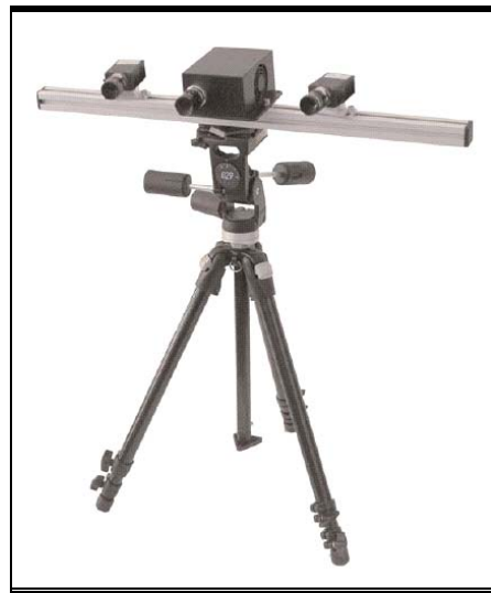
Figure 1: The scanning system: a solid bar mounted on a tripod holding a projector positioned between two cameras.
