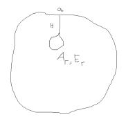
Figure 2: Inner structure for the cavity of the resonator, attached to the opening a via a one-dimensional channel.
