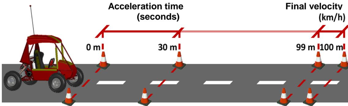
Figure 1. Illustration of the acceleration and velocity tests.
