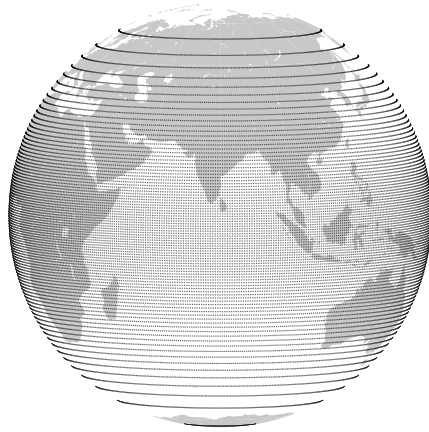
Figure 3.3: Variable resolution mesh configuration generated from the transformation corresponding to the analytic function f(z) = \ell z , \ell = 3 . This variable resolution mesh configuration has an high-resolution zone over Tropical Belt centred at the equator. The density of mesh-point distribution decreases smoothly from the equatorial belt and become coarsest at the polar regions.
