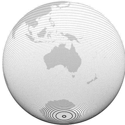
Figure 3.5: Variable resolution mesh configuration from the transformation corresponding to the analytical function f(z) = az + b , a = \frac{1}{2} , b = \frac{1}{2}ln2^2 . This variable resolution mesh configuration has a high-resolution zone over a middle latitude of southern hemisphere. The density of mesh-point distribution decreases smoothly as away from this centre. The resolution becomes coarser at both the poles.
