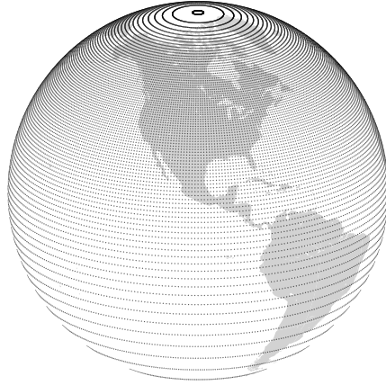
Figure 3.4: Variable resolution mesh configuration from the transformation corresponding to the analytical function f(z) = az + b , a = 2 , b = \frac{1}{2}ln2^2 . This variable resolution mesh configuration has high-resolution zone over a middle latitude of northern hemisphere. The density of mesh-point distribution decreases smoothly as away from this centre. The resolution becomes coarser at both the poles.
