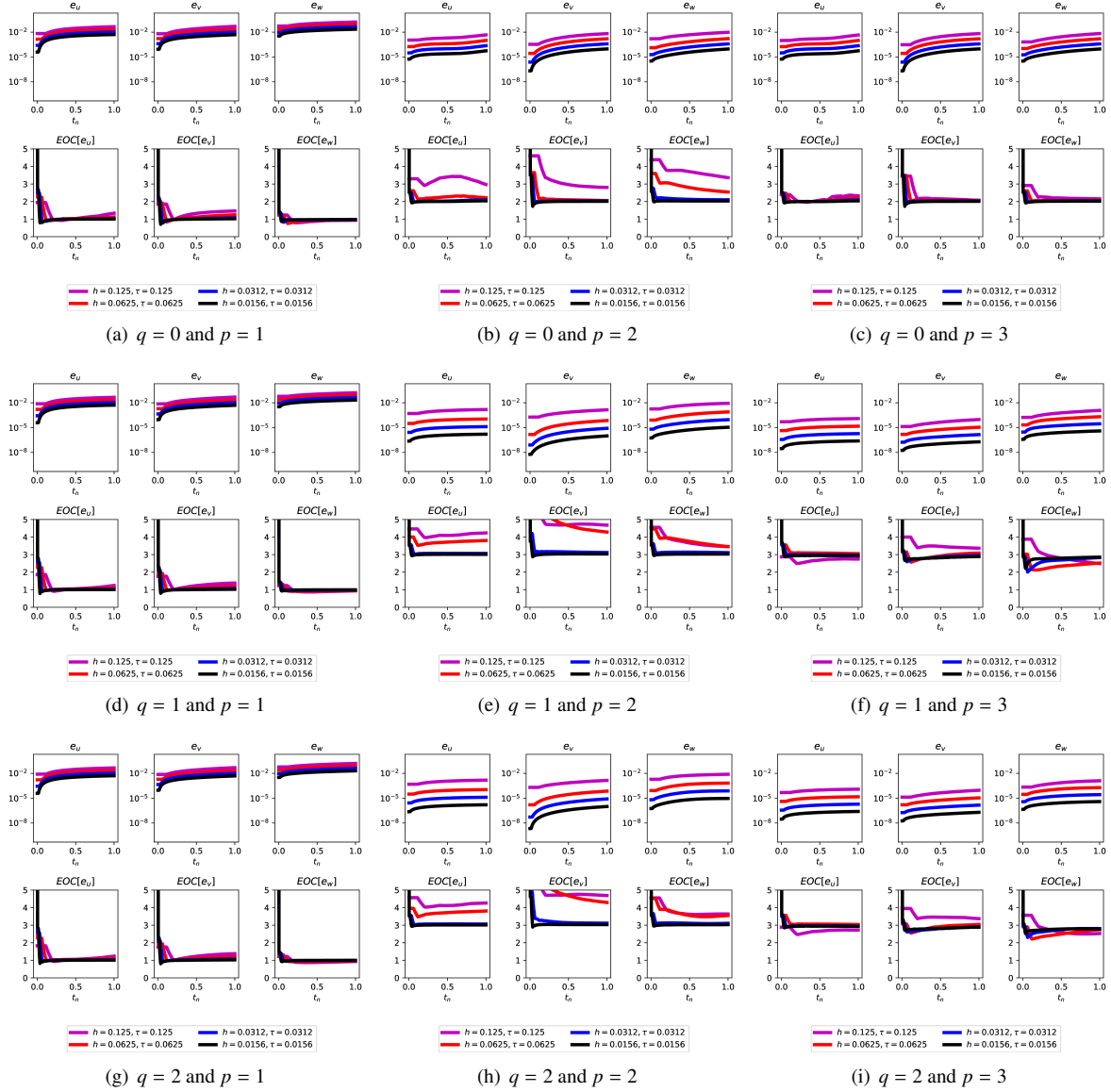
FIGURE 5.6. The error of the spatially discontinuous finite element scheme (4.1) for the nonlinear Schrödinger equation (5.11) initialised by the exact solution (5.12). Here e_U, e_V, e_W denotes the errors in the components U, V, W measured in the Bochner norm (5.2). Below we plot the EOC (5.1) corresponding to each of these errors.
