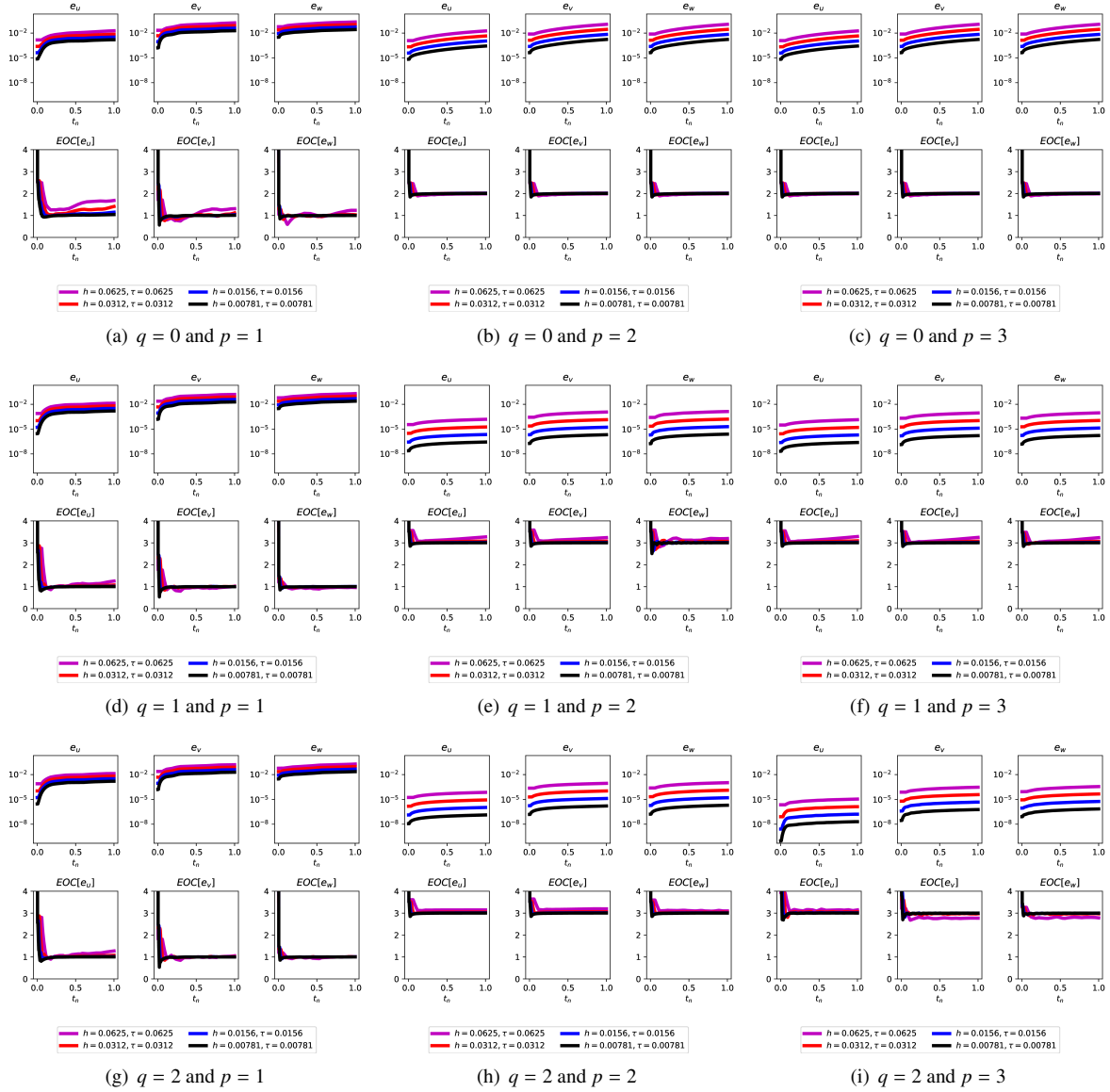
FIGURE 5.2. The error of the spatially discontinuous finite element scheme (4.1) for the linear wave equation (5.7) initialised by the exact solution (5.8). Here e_u, e_v, e_w denotes the errors in the components U, V, W measured in the Bochner norm (5.2). Below we plot the EOC (5.1) corresponding to each of these errors.
