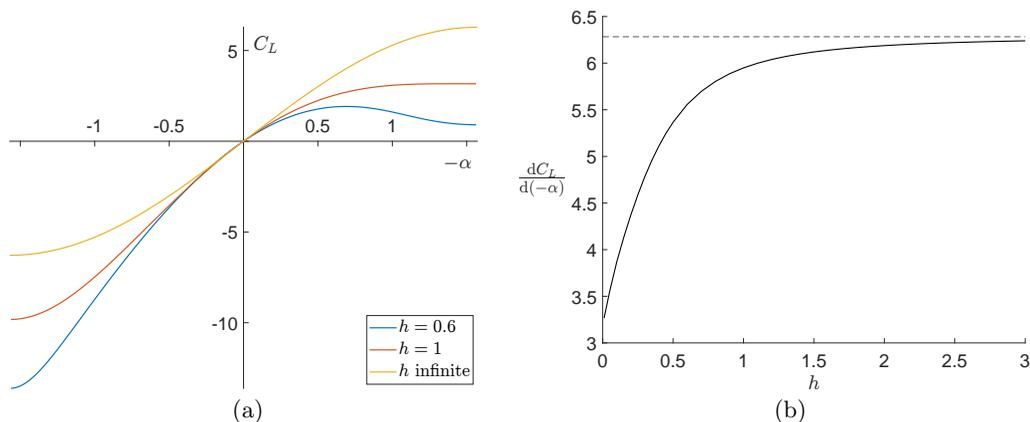
FIGURE 8. (a) The lift coefficient  $C_L$  as a function of the angle of attack  $-\alpha$  for three depths  $h$  of the midpoint of the hydrofoil. (b) The rate of change of  $C_L$  with respect to angle of attack  $-\alpha$  at  $\alpha = 0$ , as a function of  $h$ . The dashed line gives the infinite depth asymptote,  $C_L = 2\pi$ , from (6.1).
