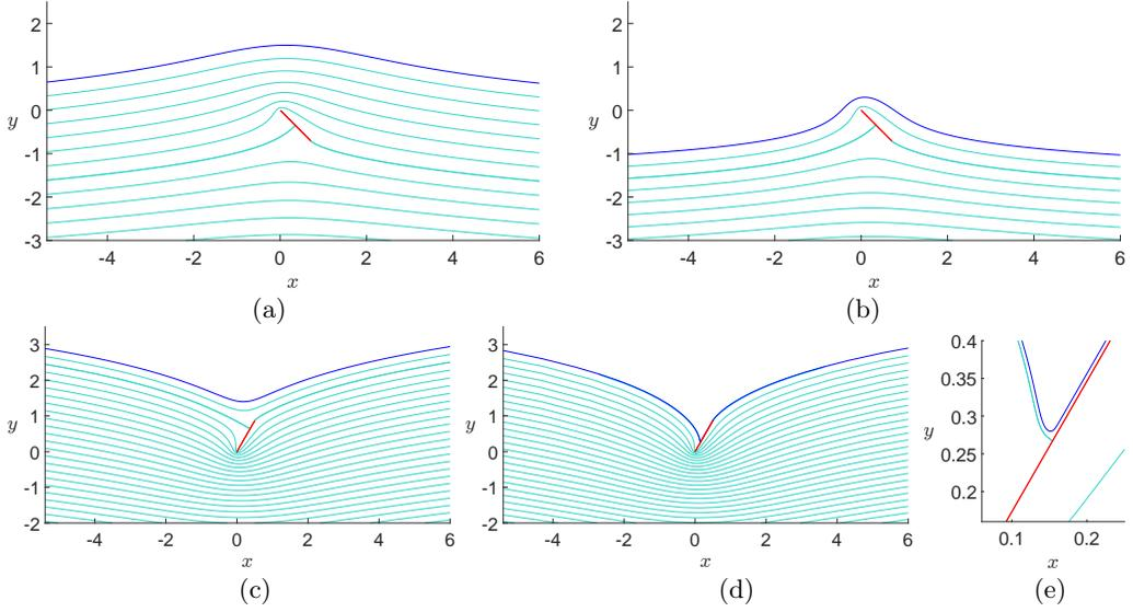
FIGURE 6. Streamlines (turquoise) for free-surface flow past a hydrofoil for various angles of attack,  $-\alpha$ , and leading-edge submergence,  $y_c$ . (a)  $\alpha = -\pi/4, y_c = 1.5$ . (b)  $\alpha = -\pi/4, y_c = 0.3$ . (c)  $\alpha = \pi/3, y_c = 1.4$ . (d)  $\alpha = \pi/3, y_c = 0.28$ . (e) A detail of part (d) near the stagnation point.
