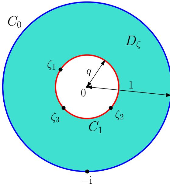
FIGURE 2. Sketch of the pre-image domain,  $D_\zeta$ , for our conformal parameterisation of the flow domain  $D$  as in figure 1.  $D$  is the image of  $D_\zeta$  under a conformal map,  $z(\zeta)$ .
