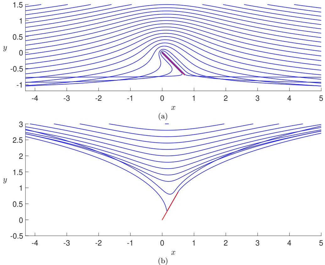
FIGURE 5. Free surface profiles (blue) for flow past a hydrofoil (red) for various angles of attack,  $-\alpha$ , and leading-edge submergence,  $y_c$ . (a)  $\alpha = -\pi/4$ ,  $y_c = 0.01, 0.05$  and  $0.1, 0.2, 0.3, \dots$  (b)  $\alpha = \pi/3$ ,  $y_c = 0.28, 0.8$  and  $1.2, 1.4, 1.6, \dots$  Lengths here and in subsequent figures are normalised on the length of the foil.
