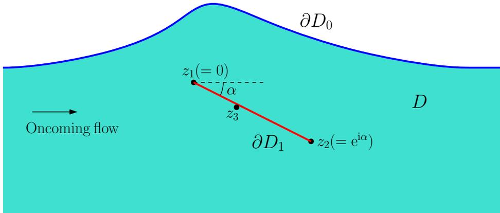
FIGURE 1. Sketch of the flow domain,  $D$ , for a free-surface flow past a submerged hydrofoil.  $\partial D_0$  denotes the free surface (in blue) while  $\partial D_1$  denotes the hydrofoil (red).  $z_1 = 0$  and  $z_2 = e^{i\alpha}$  denote, respectively, the leading and trailing edges of the hydrofoil so  $-\alpha$  gives the angle of attack.  $z_3$  denotes a stagnation point - this lies on the leading face of the hydrofoil.
