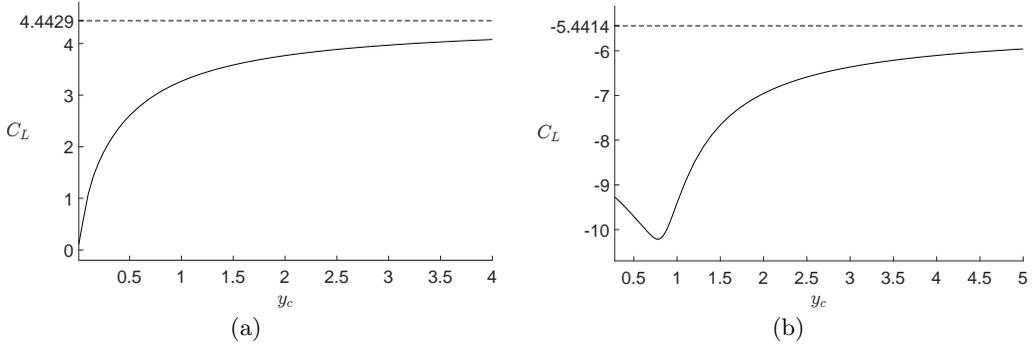
FIGURE 7. The lift coefficient  $C_L$  as a function of the leading-edge submergence  $y_c$  for the angles of attack of figure 6 : (a)  $\pi/4, (\alpha = -\pi/4)$ ; (b)  $-\pi/3 (\alpha = \pi/3)$ . The dashed line gives the limiting value for  $y_c \rightarrow \infty$  from (6.1).
